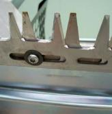
• At the end of the day give each of the grease nipples 1 pump each from a grease gun (use food grade grease). There is 1 grease nipple on each of the top and bottom gearboxes.
