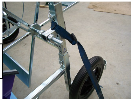
If the reel is fitted wrap the tie down around the mounting bracket as shown.
