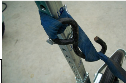
Front leg—use bolt or pin through leg for the tie down to pull against
